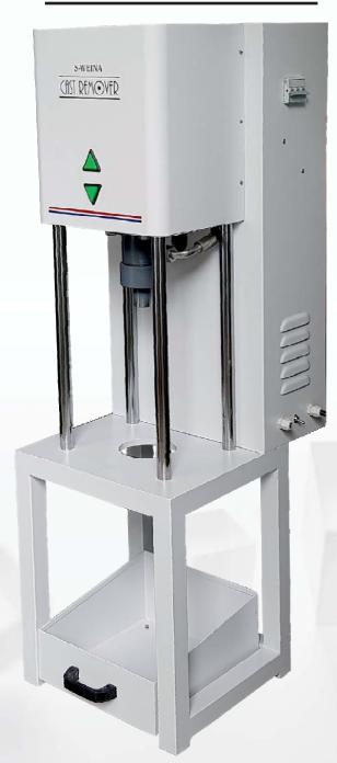
Cast Remover is a devices to reduce the investment from the Casting Flask after the casting process. Powerful Hydraulic Piston pushes the casting away from the flask leaving the flask cylinder untouched.
